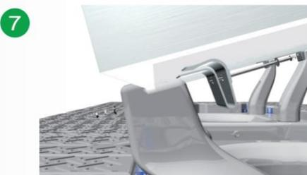
Using Clamp Kit and Screw Kit to fix solar panel on the Front Legs.
